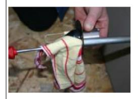
Clean residues off air cover using a brass wire brush. Clean flicker detector tubes.
