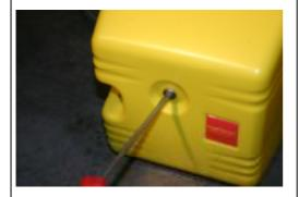
Use screwdriver to loosen the fastening bolt on the C1 burner hood and remove burner hood.
