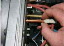
**Compressor air supply coupling:** Press ring towards the back and pull off.
