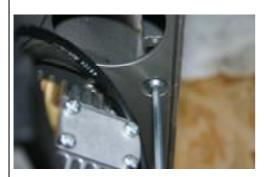
Loosen four cheesehead bolts on burner housing and remove housing lid.
