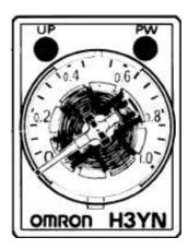
To undertake service work on the operationally warm burner, the settings wheel can be turned to the right until it hits the stop. This reduces the startup delay to 1 min..
