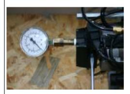
Pressure setting on the Suntec oil pump is realized parallel to setting of the output and measurement data. This is done on the right side of the upper edge of the oil pump with a large flat-blade screwdriver.
